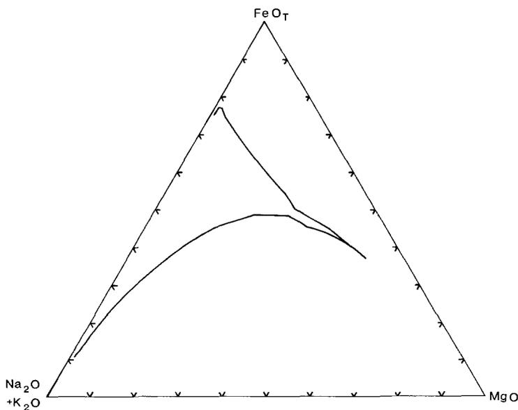
**Fig. 15.** Calculated liquid paths for the fractional (upper curve) and equilibrium (lower curve) crystallization of an olivine boninite (U 1, Irvine and Sharpe 1982) along the QFM buffer at 1 bar. The crystallization interval was taken to be 25° C and results at each temperature are shown connected by solid lines.  $FeO_T$  denotes the total iron content of the melt expressed at FeO. The diagram is in wt %
