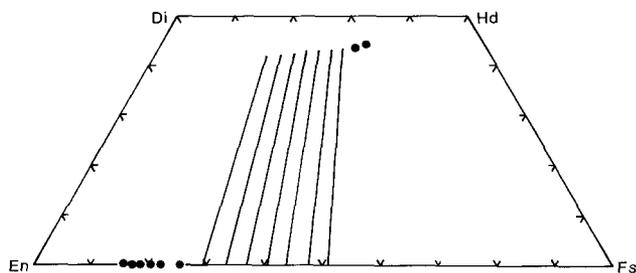
**Fig. 17.** Calculated pyroxene compositions precipitated during the fractional crystallization of an olivine boninite (U 1, Irvine and Sharpe 1982) along the QFM buffer at 1 bar. The crystallization interval was taken to be 25° C and results at selected temperatures are shown. Coexisting pyroxene compositions are linked by lines rather than being denoted individually by solid circles. The diagram is in mole %
