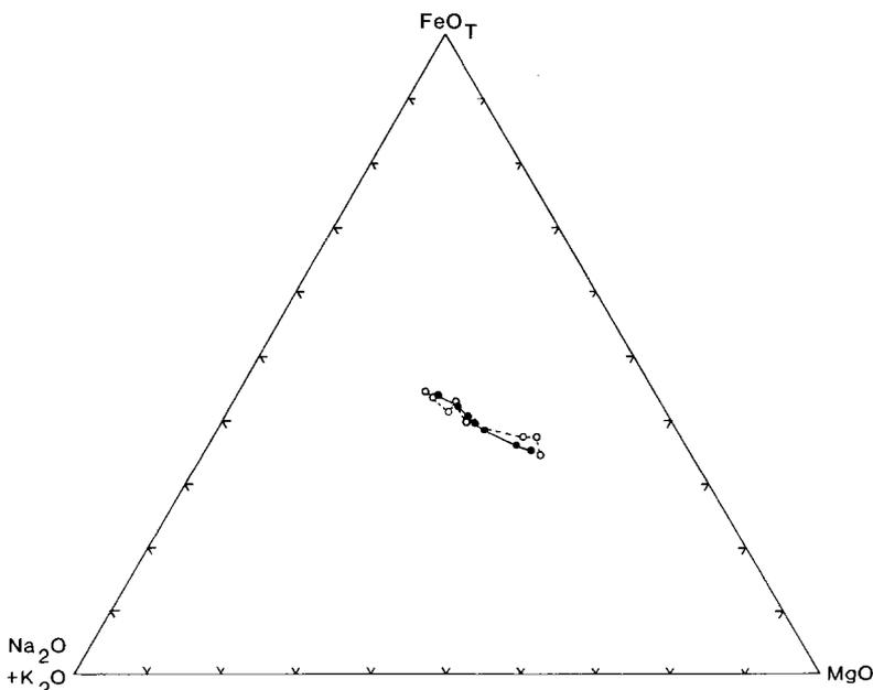
**Fig. 3.** Calculated liquid path for the equilibrium crystallization of a basaltic andesite (JOR 44, Table 1) along the Ni–NiO oxygen buffer at 1 bar. Solid lines link the calculated results obtained at 1,254° C (lower right), 1,227°, 1,185°, 1,175°, 1,165°, 1,150°, and 1,140° C (upper left). Corresponding experimentally determined liquid compositions (Mo and Carmichael 1985) are joined by dotted lines.  $\text{FeO}_T$  is the total iron, expressed as FeO, in the liquid. The diagram is in wt %
