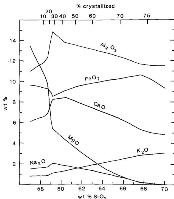
**Fig. 16.** Calculated liquid variation diagram for the fractional crystallization of an olivine boninite (U 1, Irvine and Sharpe 1982) along the QFM buffer at 1 bar. The crystallization interval was taken to be 25° C and results at each temperature are shown connected by solid lines. Note the wt % crystallization scale which labels the top of the diagram.  $\text{FeO}_T$  denotes the total iron content of the melt expressed at FeO
